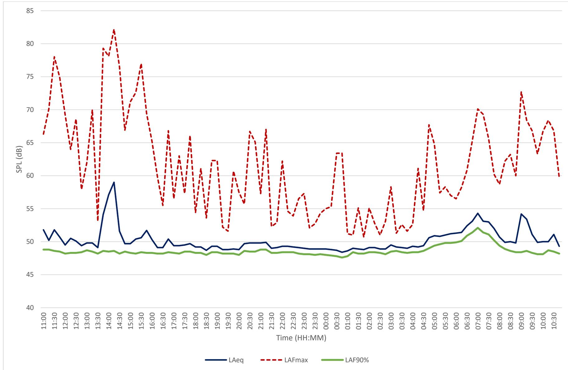
Figure B.6 – Most Commonly Occuring Background Noise Level at Position A
