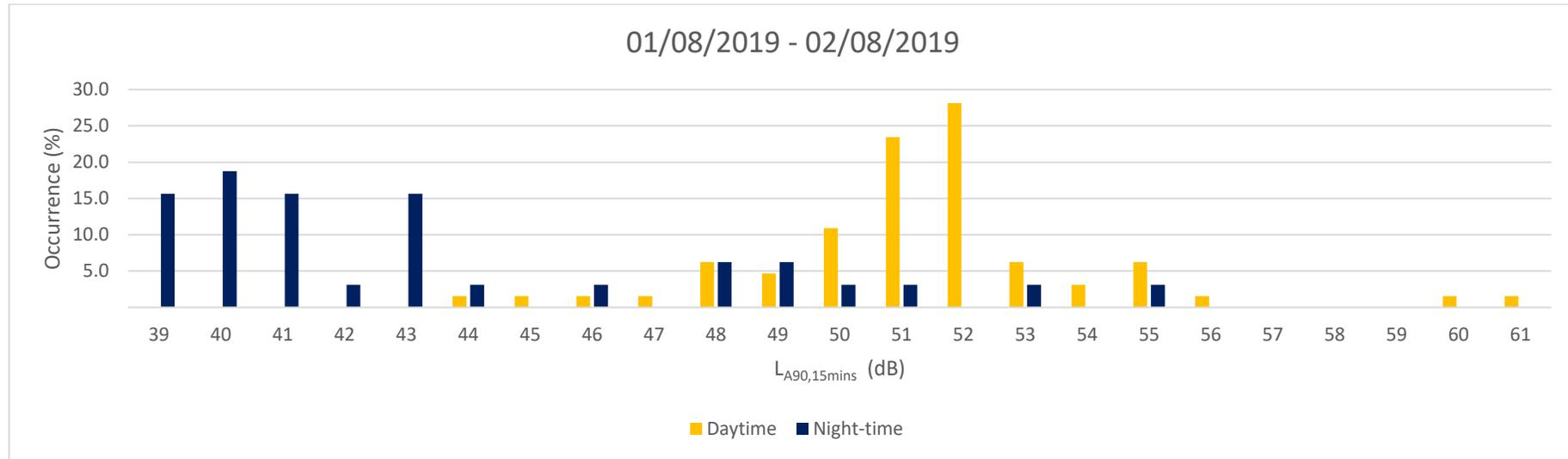
Figure B.7 – Most Commonly Occuring Background Noise Level At Position B
